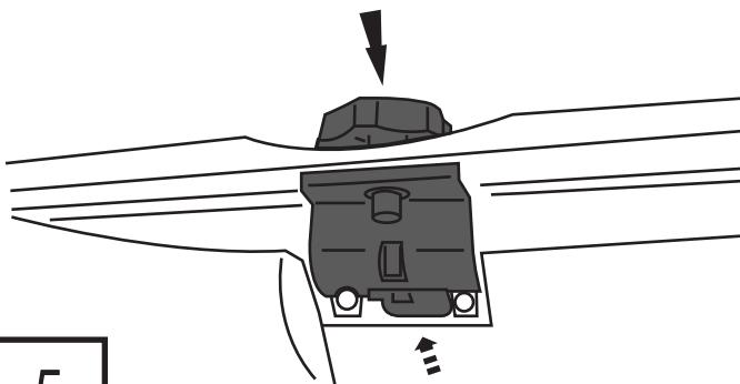
Wrap the 2 straps attached to the main section of fabric around the rear-middle of the sound bar. Insert plastic hooks into the holes on the underside of the sound bar. Tighten the strap until snug.
