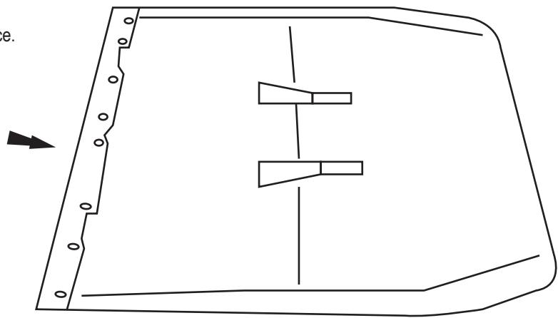
Lay the header channel on top of the fabric tucking inside and secure with snaps as shown.
