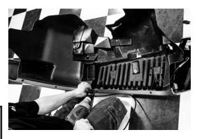
Seperate fender flare from splash shield. Reinstall splash shield only on fender, prior to marking for cutting.
