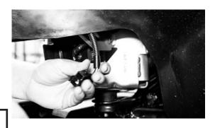
Starting at the front of the fender flare, pull to remove the flare and splash shield assembly from the vehicle fender. **NOTE**: You may notice loud popping noises as clips release, this is normal.
