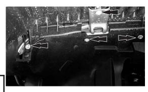
Remove (2) additional factory bolts from inside of splash shield. Save bolts.
