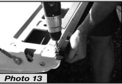
■ Install the remaining self-tapping screws, making sure to provide even spacing between them.
