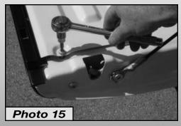
**G**■ With the Tailgate Extrusion secured, carefully close the tailgate, being cautious not to strike the ends of the Tracks.
