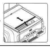
Spray 303<sup>®</sup> on a rag and wipe the top gasket in the Track back and forth.
