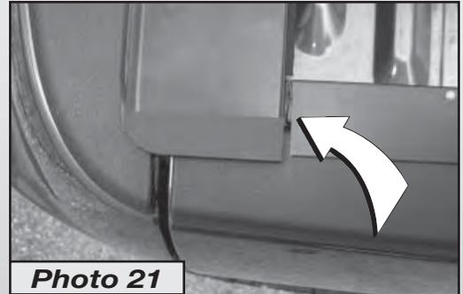
toward the tailgate (**Photo 20**) so that the Track End Caps contact the inside surface of the tailgate. Make sure the Track End Cap metal blocks contact the Tailgate Extrusion End Caps (**Photo 21**). **Note: If the Tracks are not positioned as shown, the Latch Mechanism will not function correctly.**
