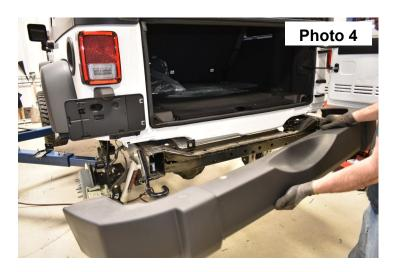
4. Using a 18mm socket, remove the stock tow hook. See Photo 5 & 6.
