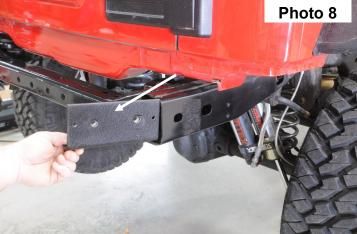
Position the bumper on the frame and secure with the 12mm x 40mm bolts, lock washers and flat washers. See Photo 9.
