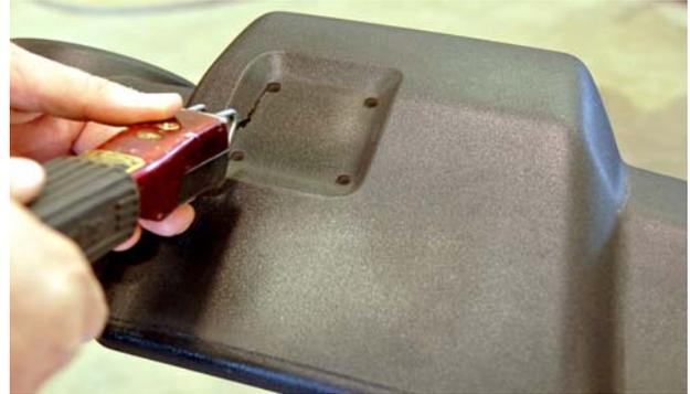
13. Reinstall bumper, using the studs from the new bumper bracket, and supplied 12mm-1.75 nuts. Tighten using a 19mm socket.
