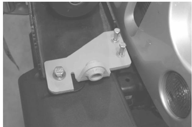
20. Install the d-rings on the d-ring mount as shown in **Photo 13**.
