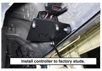
8. Connect the corresponding electrical connectors of the main harness to the controller. Photo 7 / 8
