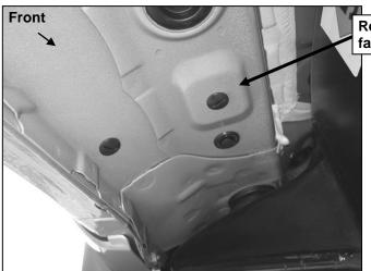
Remove plastic plugs or factory hex bolts (if equipped)
