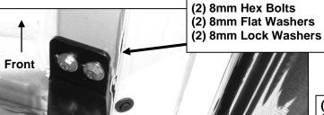
(Fig 2) Driver side front mounting location pictured
