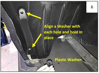
In one of two holes at front of wheel well, reach behind sheet metal and hold a supplied plastic washer behind factory hole in sheet metal (aligned with hole in wheel well liner).
