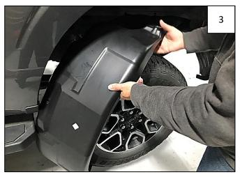
Slide the Rear Wheel Well Liner behind wheel at rear of vehicle. It is helpful to tilt the liner at a 45-degree angle at front of wheel and then straighten it out once it's behind the wheel.
