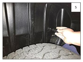
Start a supplied Truss Head Screw through each hole in back of wheel well liner and into clips installed in Step 1. Tighten both screws.
