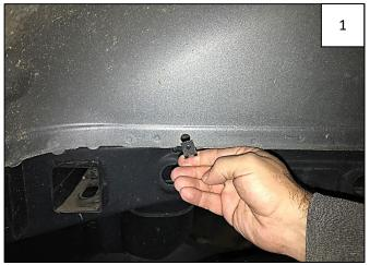
Install 2 supplied "U" Clips over factory holes at back of rear wheel well, as indicated in next step. Flat side of clip will face *out* when clip is installed.
