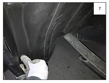
While holding Plastic Washer at inside of sheet metal, insert a supplied Plastic Retainer through hole in wheel well liner, factory hole in sheet metal, and into Plastic Washer. Repeat Steps 6 and 7 for upper hole at front of wheel well.
