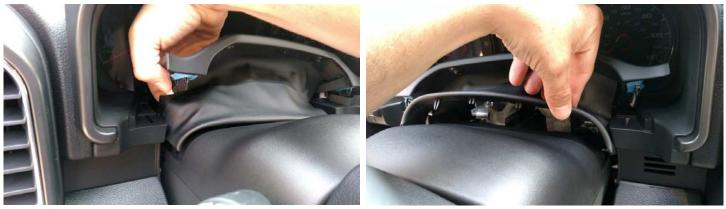
6. Raise steering column up to the highest position and reach behind the kick panel on the left and right side of the column and pull towards you to disengage the upper retaining clips. This allows access to the screws that retain the I/C Shroud.
