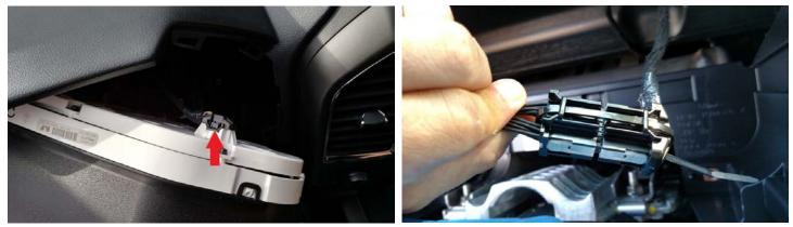
12. For the F150, tuck the harness and module on top of the air duct that runs inside of the I/C cavity to gain clearance for installation. For the F250, access to the top of the duct is limited so insert the harness and module below and orientate them sideways.
