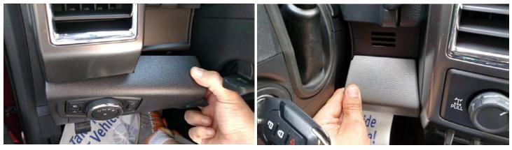
7. With the kick panel lowered, remove the (2) 7mm screws that retain the I/C Shroud.
