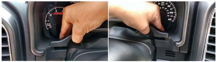
5. Next disconnect the vinyl column cover from the steering column itself. Reach under the backside of the cover and gently pull up, it will disconnect from the steering column rather easily. Completely remove this piece.
