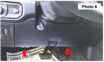
8. Pull the panel toward the rear of the truck to release the tabs holding the panel in place.
