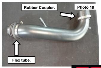
19. Install the intake / Rubber coupler onto the throttle body of the engine. Secure the rubber coupler using (1) of the supplied 3" clamps. See Photo 19 & 20.
