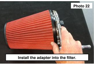
22. Install (1) 3" clamp around the flex tube. Then install the filter adapter into the flex tube, pushing the adapter against the heat shield and the flex tube to the adapter. Then tighten the clamp using a 8mm socket. **See Photo 23 & 24.**
