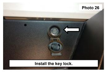
30. Make sure the key lock sits snug onto the backing plate of the bumper. See Photo 27.
