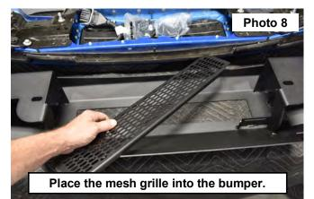
10. Secure the mesh grille using the driver and passenger side brackets and secure the grille using the supplied 8mm Bolts, 8mm Flat Washers and the 8mm Nuts. Tighten using a 13mm wrench and socket. See Photos 9 and 10.
