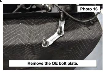
16. Support the bumper. Install the OE bolt plate into the bumper and install the bumper onto the vehicle and secure using the OE retained nuts. See Photos 17 and 18. <u>Pic shown for vehicles without factory receiver hitch. If factory hitch is present, the stock three bolt nut plate will install into the hitch bracket and secure to the bump-</u>
