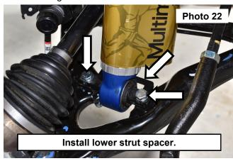
tained bolt tighten using a 13mm socket. See Photo 23.
