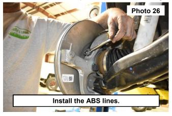
18mm socket. Install the brake line onto the knuckle using the retained bolt. Tighten using a 10mm wrench. **See Photo 27.**
