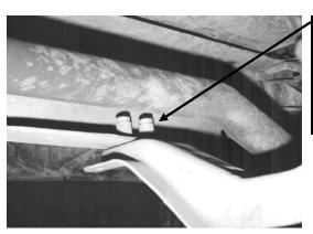
The sleeves may be either on top of the frame rail or on the bottom from the factory as shown here.
