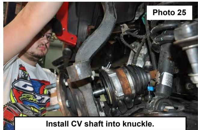
spindle. **Use the supplied 1/2" washer from 54531BAG2, place between knuckle and nut. See Photo 26.**
