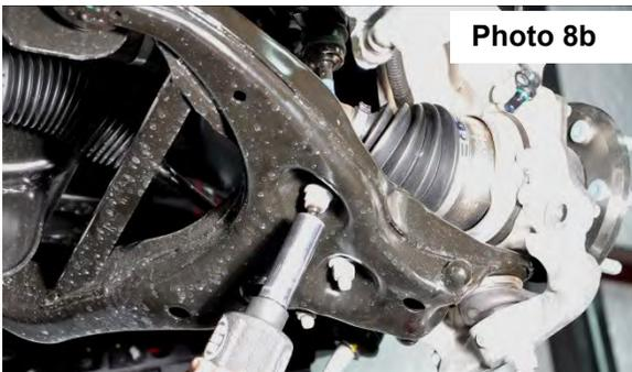
**Remove the lower strut bolts. 14-20 Models**
