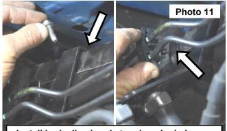
Install brake line bracket and push pin brace.
