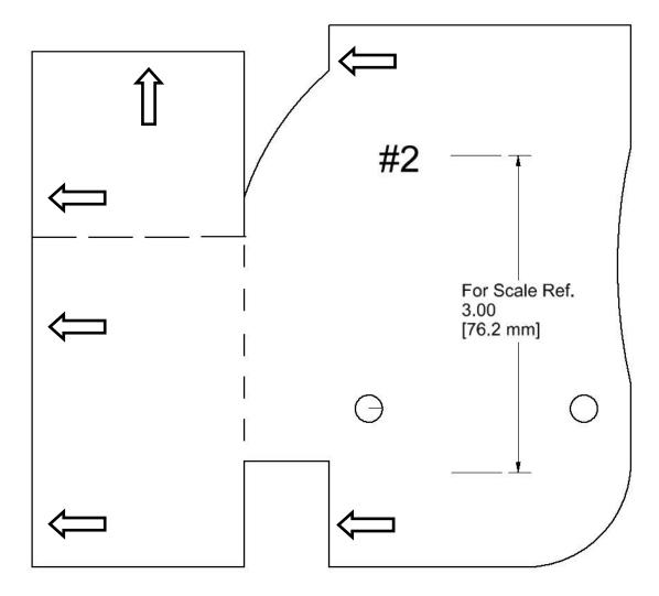
Mark at arrows when template is on the vehicle.
