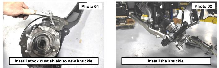
60. Install the knuckle to the upper ball joint using the stock hardware. See Photo 64.
