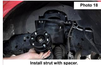
21. Reassemble the suspension in reverse order of tear down.
