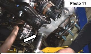
Remove lower ball joint using 21mm.
