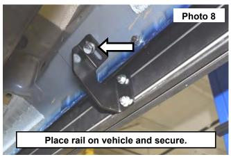
10. Secure the rail to the pinch weld using (2) of the supplied 8mm x 50mm bolts (2) 8mm flat washers and (2) 8mm flange lock nuts. See Photos 9 and 10.
