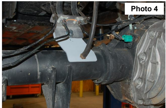
7. Using a 24mm socket, remove the stock u-bolts. Use the floor jack to lower the axle assembly to allow for lifted block installation.
