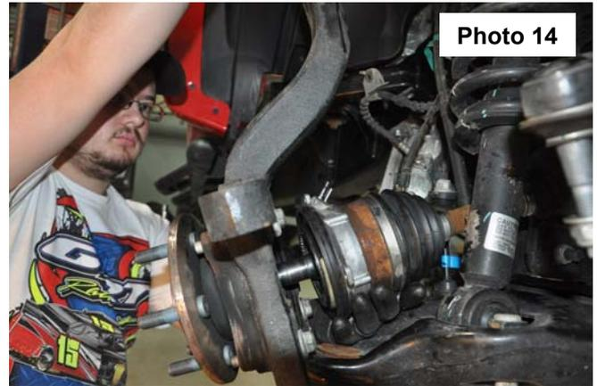
17. Using a floor jack, raise the lower control arm and connect the upper ball joint on the upper control arm to the spindle. Using a 21mm wrench, torque to manufacturer specs. If ball joint turns while tightening, use a 3/8" wrench to hold the ball joint.
