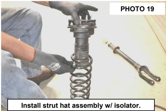
28. Place the strut and coil assembly in the strut compressor, compress the strut, and install the factory top nut using an 18mm socket.
