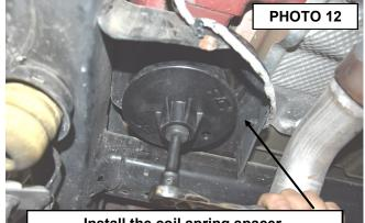
Install the coil spring spacer.
