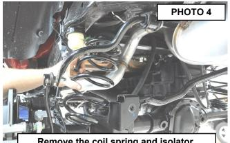
Remove the coil spring and isolator.
