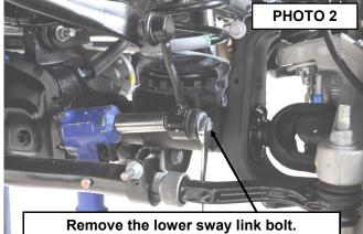
pull down on the shock to remove the bolt. See Photo 3. Retain stock hardware.
