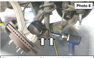
Remove lower strut. 21mm on bolt / 24mm on nut
