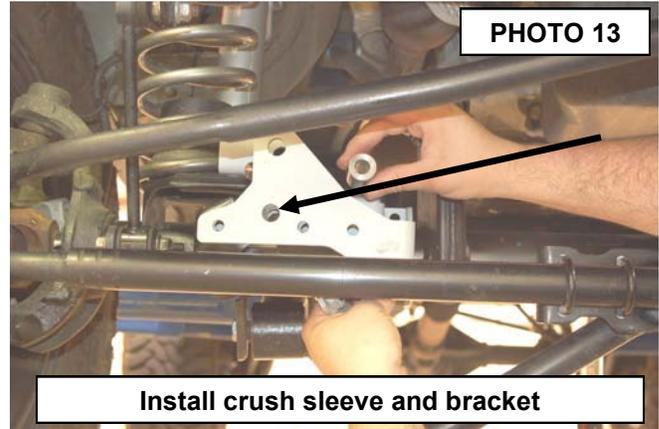
24. Install the stock hardware in the bracket as shown. **See Photo 14**. Do not tighten at this time.
