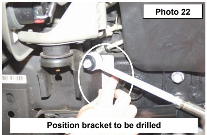
**Position bracket to be drilled**
