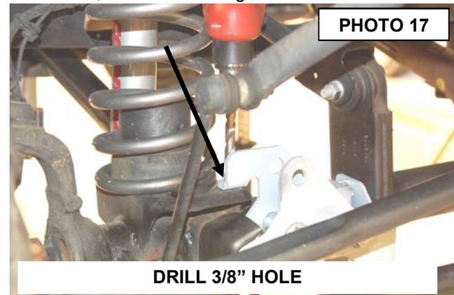
28. Tighten all 3/8" hardware using a 9/16" wrench.
