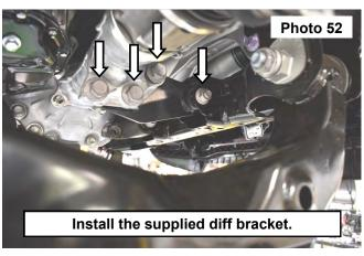
52. Install the diff bracket spacer and diff bracket beneath the diff using stock hardware at the frame and supplied 14mm x 65mm bolts and (2) 14mm flat washers in the diff using a 22mm socket/wrench.
