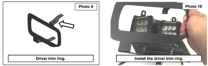
ers and (2) 1/4-20 nylock nuts. Tighten using a 3/16 Allen wrench and a 7/16" wrench. See Photo 10 and 11.
