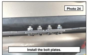
16. Your rack should look like this at this time with front and rear panel bolted to the side rails, and the bolt plates installed. All mounting hardware should still be loose. **Photo 25 / 26**
