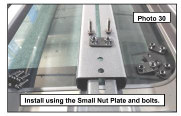
19. Attach one of the tie downs to the front panel middle mounting holes using the 8mm button head bolts, washers and small nut tab. Tighten down. Hook a ratchet strap to the tie down hole and pull all the way to the back of the rack. This will be your guide to center the cross rails. Once you have the strap in place, center the cross rails and torque the mounting hardware. You can leave the tie down there or move it to where it is needed. Photo 31 / 32
