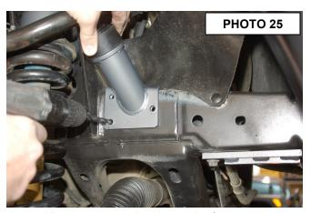
three holes in the frame. Use the self-tapping 3/8" x 1" bolts in 1770Bag9 to secure bracket to the frame.
