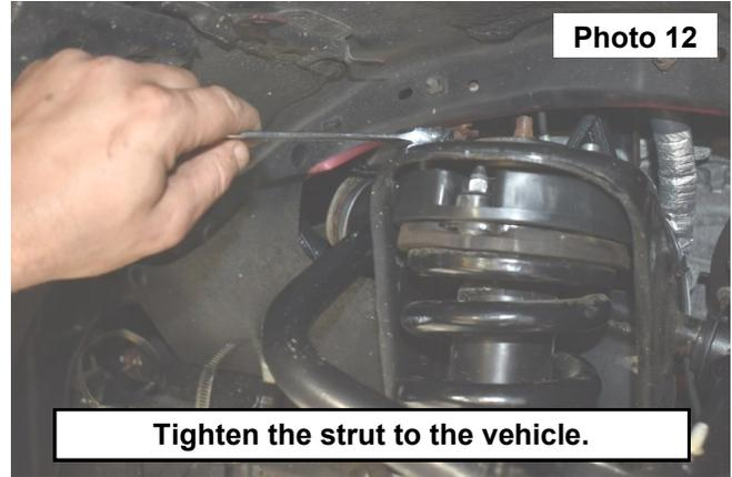
13. Position the strut assembly to reinstall the lower strut bolt in its original position that it was removed. Using original hardware and a 19mm socket torque to 100ft lbs.
