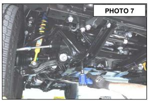
10. Measure 1" up and 4.5" from the rear of the skid brace. See PHOTO 8 & 9.
