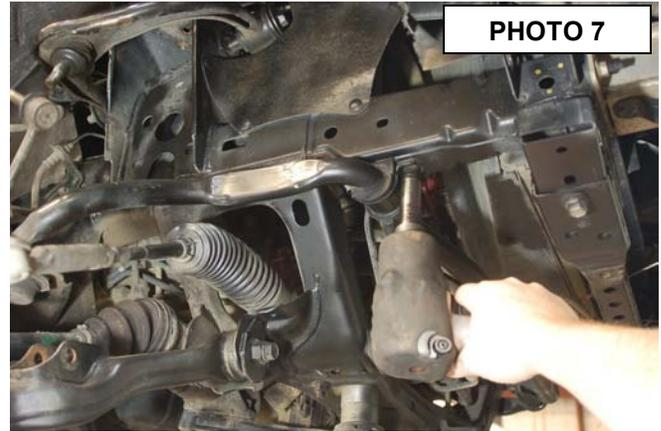
19. Remove the lower control arm with a 19mm socket and wrench. **See Photo 8.**
