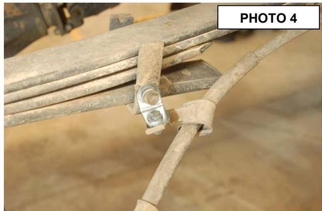
12. On the driver side of the rear axle bolt the rear brake extension bracket to the axle using factory hardware and a 12mm wrench. Attach the factory bracket to the new extension bracket using the supplied 1/4" bolts, washers, and locking nuts. Tighten with a 11mm socket and wrench. **See Photo 5.**
