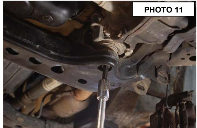
26. Starting from the edge of the cam bolt plate on the back side of the rear cross-member make a mark at 3" and another mark at 12". This is where the rear cross-member needs to be cut to allow the diff to drop down. **See Photo 12.**
