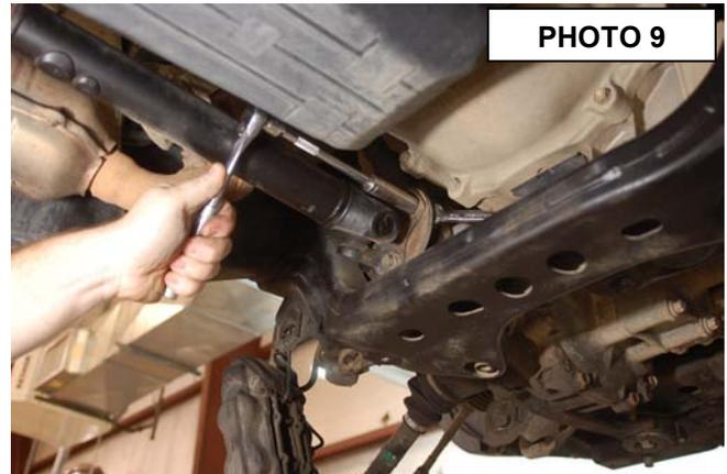
22. Unplug the vent tube and remove the diff actuator using a 12mm socket. Remove the actuator wires from the diff on the passenger side. Unplug and remove the vent tube from the top of the diff using a 12mm socket.
