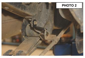
1/4" bolts, washers, and locking nuts to attach the factory mount to the new bracket.
