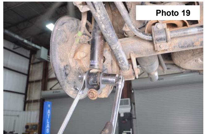
15. Tighten lower mount bolt using a 17mm wrench, torque to 71 ft. lbs. **See Photo 20.**
