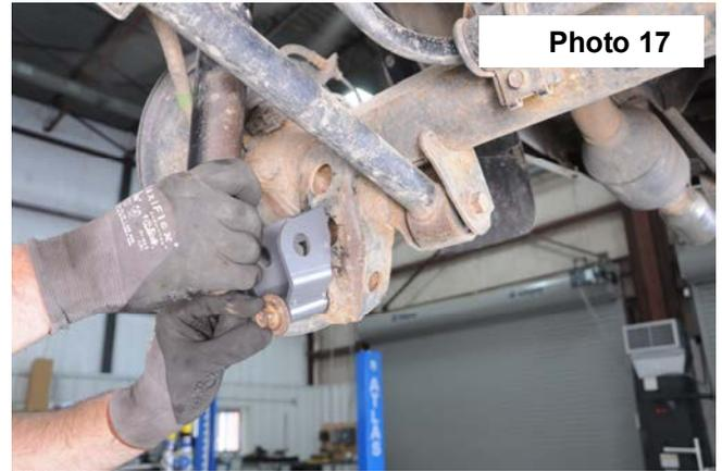
13. Place supplied 3/8+bolt into upper hole on shock bracket. **See Photo 18.**
