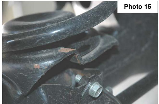
9. Using a 12mm wrench, reinstall the brake line bracket on the drivers side, and ABS bracket on the passengers side.
