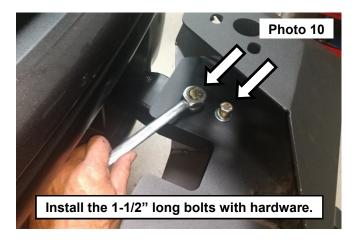
14. Torque the 10mm bumper bracket hardware to 45 ft-lbs. Then torque the 12mm bolts under the bumper bracket
