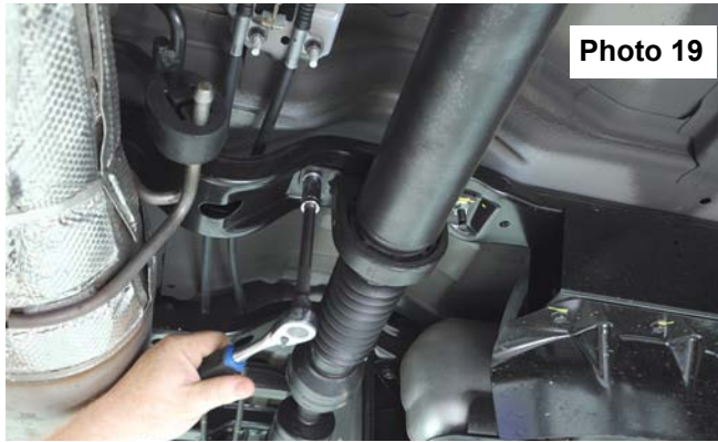
Lower the carrier bearing.
