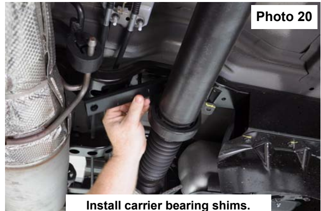
Install carrier bearing shims.
