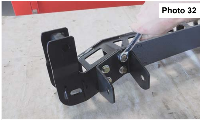
Install differential drop brackets on front crossmember.
