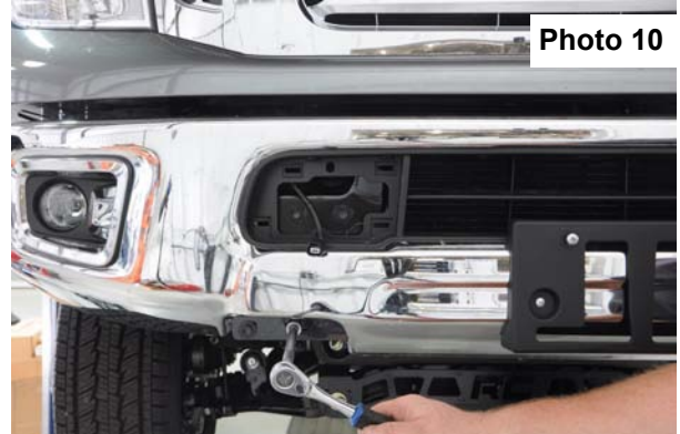
Remove the front bumper mounting bolts.
