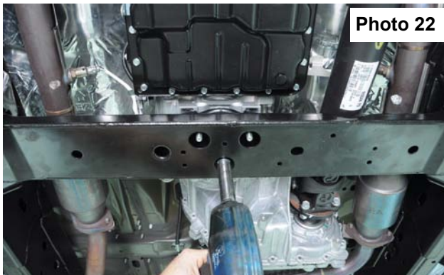
Remove transmission mount nuts.
