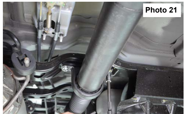
Tighten carrier bearing bracket.
