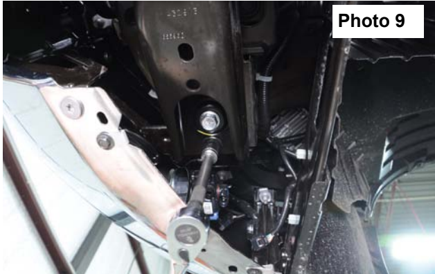
Remove the lower bumper mounting bolts.
