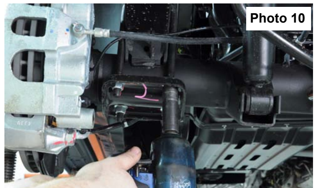
Remove the factory u bolts and hardware.
