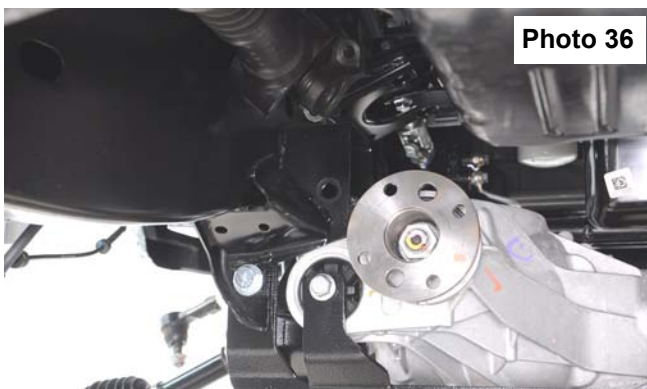
Bolt rear crossmember to differential.
