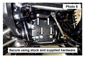
7. Install the winch to the mount using the hardware supplied with the winch. See Photo 9.
