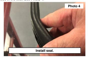
5. Use a dead blow hammer to fully seat the seal. See Photo 5 and Photo 6.
