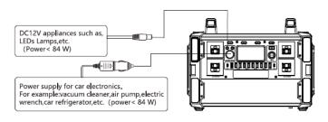
Note: The working range of DC output voltage of this product is 12V (regulated voltage), and the maximum output current is 7A.
