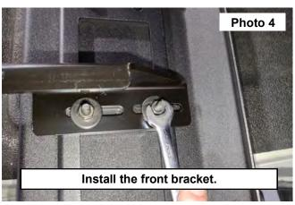
Repeat the installation of the (2) bolt plates in the slot for the center and rear step mounting brackets. See Photo 5.
