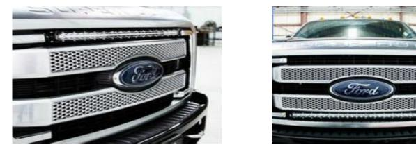
Or, combine 2 kits and double your light output by mounting one light on top and one on bottom as shown.
