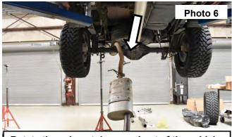
Rotate the exhaust down and out of the vehicle.
