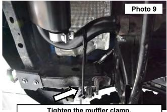
Tighten the muffler clamp.
