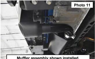
Muffler assembly shown installed.
