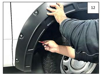
Hold flare to vehicle and mark 1 flare hole location with grease pencil.
