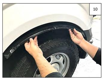
Line up the holes in the Inner Bracket with the 3 uppermost factory holes, installing correct Inner Bracket for each side.
