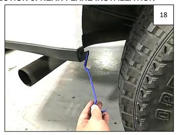
Using a pry tool, remove plastic factory fastener from rear of wheel well.
