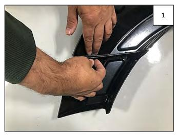
Install Extension Pieces to main front flares using 2 supplied #8 Speed Clips and #8 Screws per side.
