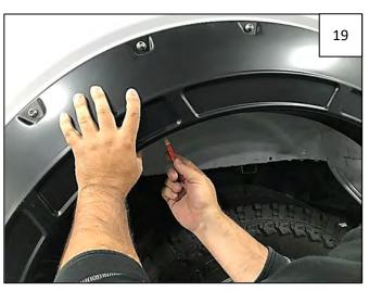
Hold flare to vehicle and mark 4 flare hole locations with a grease pencil.
