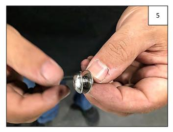
Install a supplied SS Pocket Washer onto each SS Pocket Torx Bolt.
