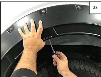
While holding flare to vehicle, start supplied #10 Truss Screws through the 4 topmost mounting holes in flare and into clips installed in Step 22.
