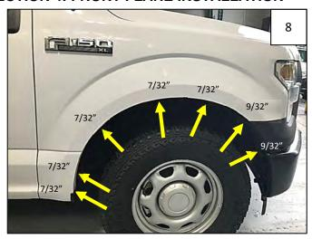
Remove 5 factory screws with a 7/32" Socket. Remove 2 front-most factory screws with 9/32" Socket. Retain Screws for reinstallation. **NOTE**: For Platinum Edition, additional screws will need to be removed and saved for reinstallation.
