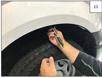
Using a 7/32" Socket, reinstall 3 top factory screws through the holes in the Inner Bracket. Tighten screws.
