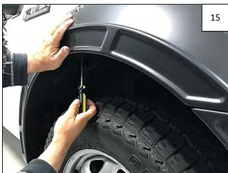
Position flare on fender, applying pressure on flare toward vehicle surface. Line up the flare mounting holes with the mounting clips on the Inner Bracket. Using a Phillips Screwdriver, install 3 supplied #10 Truss Screws through the flare and into clips. Do not tighten.
