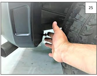
Install supplied Nylon Retainer through flare and into factory hole at rear of wheel well.
