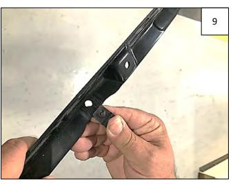
Attach 3 #10 "U" Clips to each Inner Bracket over predrilled holes as shown. **NOTE**: Driver Side Inner Bracket is marked with an "LF" and Passenger Side Inner Bracket is marked with an "RR."
