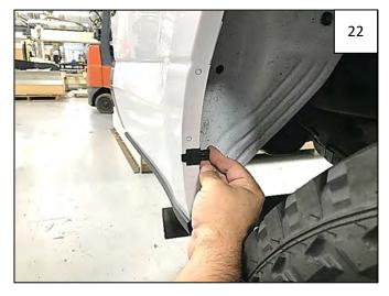
Install a supplied Long "U" Clip over each Foam Tab.
