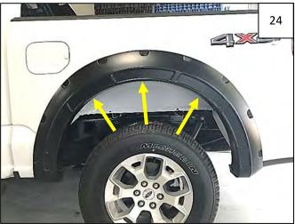
Install 3 supplied Truss-Head Screws through upper holes in flare and into clips installed in Step 22. Apply pressure to flare towards vehicle body at each fastening point and tighten all fasteners.
