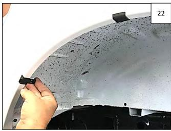
Slide a supplied Long "U" Clip over each foam tab. Clip will overhang wheel well lip on both inner and outer surface. Clip hole should be centered approximately over mark made in Step 19.
