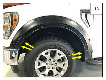
Still pressing flare firmly to fender, reinstall 4 remaining factory screws removed in Step 5. Apply pressure to flare towards vehicle body at each fastening point and tighten all fasteners.
