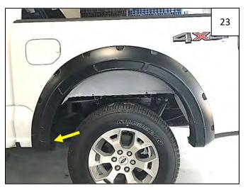
While holding flare to vehicle, start 1 factory screw in lower front of wheel well.
