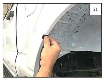
Peel backing from supplied Foam Tab. Center a Foam Tab over each mark made in Step 19, folding each tab over the wheel well lip. Press to adhere.
