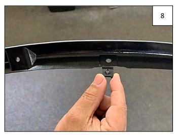
Install 3 Short "U" Clips onto the Inner Bracket as shown. NOTE: Driver's side Inner Bracket is marked with an "LF" and the passenger's side Inner Bracket is marked with an "RF".
