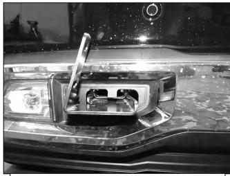
(Fig 11) Passenger/right side Bracket installed
