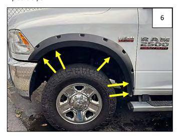
Align flare with vehicle. Start 5 factory screws through holes in flare and into factory holes.
