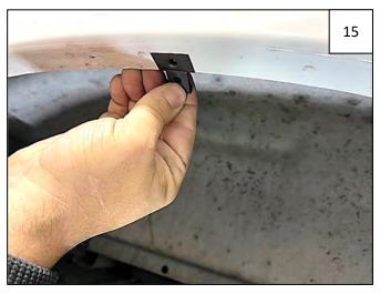
Slide a supplied "U" Clip over the mounting tab centering over the hole made in Step 14.
