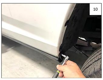
Using an 8mm socket, remove and retain factory screw at front of rear wheel well.
