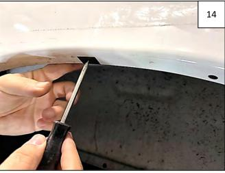
Using an awl, pierce Mounting Tab into the factory hole underneath.
