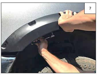
Press inward on flare to apply pressure to the flare and tighten all screws.
