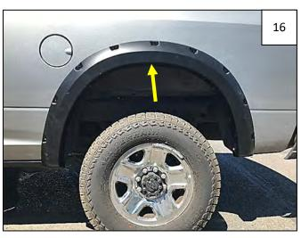
Align flare on fender. Using a Philips screwdriver, start supplied Truss Head Screw through flare and into clip installed in Step 15.
