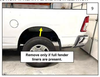
If vehicle is equipped with full fender liners, remove top most factory screw at top of fender; retain for reuse. If vehicle is not equipped with fender liners, proceed to Step 10.
